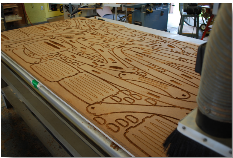
Parts 'Nest' together, Minimizes Waste.
